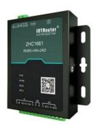
ZHC1661 is a network IO product that supports 4 channels of analog detection (current 4~20mA), 2 channels of analog output (current 4~20mA) and one serial port transparent transmission, compatible with Modbus RTU/TCP protocol. With "remote control" as the core function, it is highly usable, and users can easily and quickly integrate it into their own systems to realize remote, local area network and local control based on Ethernet and RS485.
