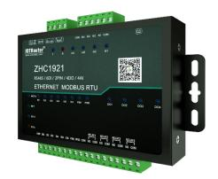
ZHC1921 is a network IO product that supports 6 channels of dry (wet) node detection, 4 channels of relay (COM, NO) output, 4 channels of analog (current 4~20mA) detection, and one serial port transparent transmission. It is compatible with Modbus RTU/TCP protocol. With "remote control" as the core function, it is highly easy to use, and users can easily and quickly integrate into their own systems to realize
