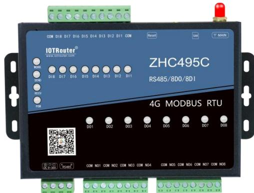
ZHC495C is a support 8 Road dry (wet) node detection, 8 Road relay (COM, NO) output, 1 channel RS485 transparent transmission network IO products, compatible with Modbus RTU/TCP protocol. With "remote control" as the core function, it is highly easy to use, and users can easily and quickly integrate it into their own systems to achieve LTE, RS485 remote and local control.
